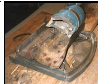
Finite Element Analysis is used to model rupture in a support fixture
