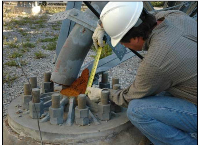
Field and laboratory fracture examinations are conducted to determine origin and cause of failure
