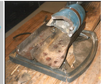
Support Fixture in which a 105 mm Projectile Accidentally Exploded
