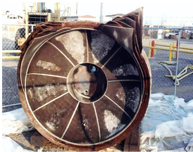
Figure 1. Failure of a urea reactor and release of the vessel head.
