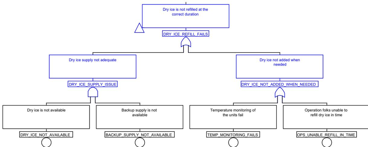
**Figure 4. Dry Ice Refill Failure**
