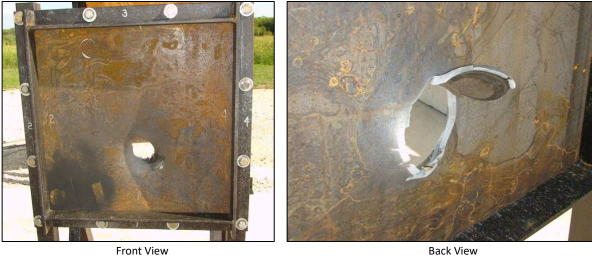
Figure 3. Projectile Perforation of a Steel Plate
