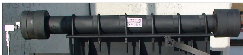
Figure 2. PTRC Test Pressure Vessel
