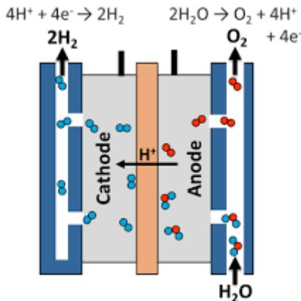
Figure 2. Typical Electrolyzer Operation (Courtesy: Department of Energy)
