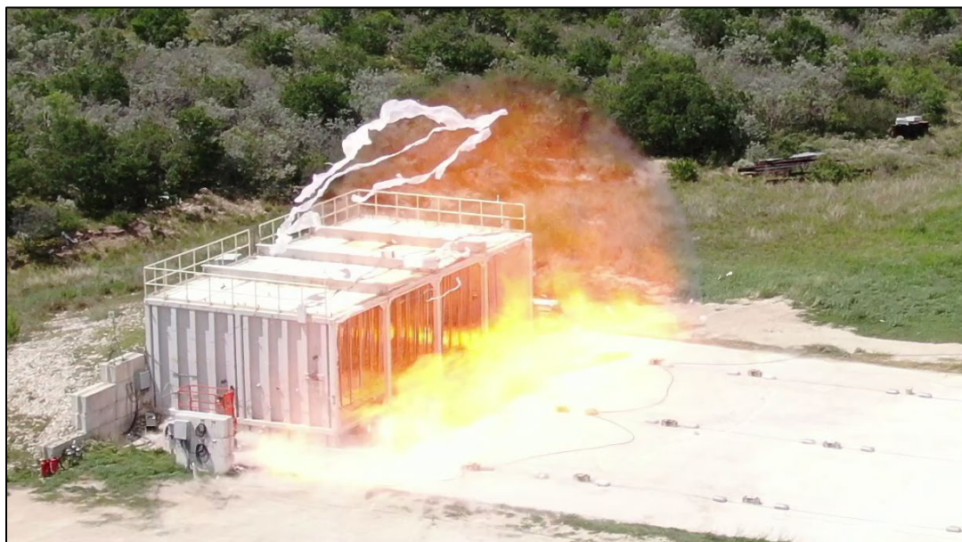
Figure 3. Still frame of a vented hydrogen/methane VCE from BakerRisk's Deflagration Load Generator
