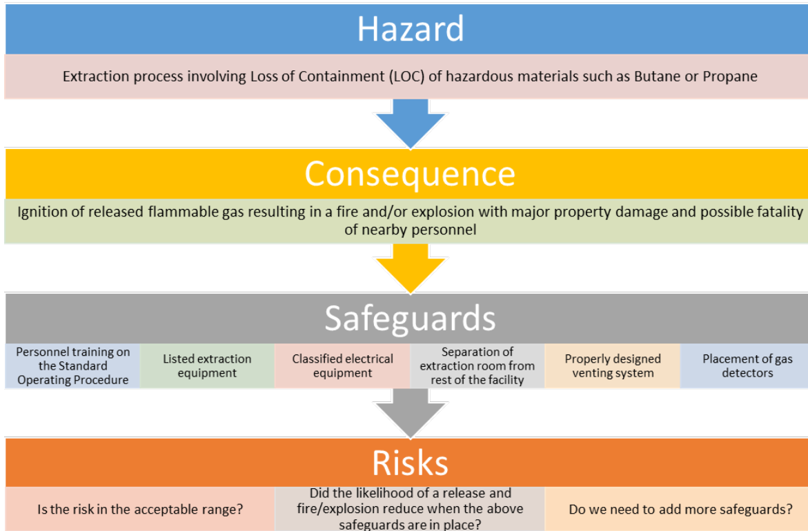
Figure 3. A simplified HIRA flow chart for an Extraction Process
